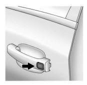
When all doors are closed and the ignition is off, the vehicle can be locked by pressing this area on the door handle. This feature will be available for several minutes after the vehicle has been turned off.
